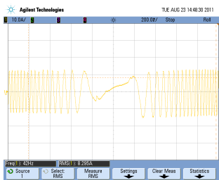
FWD/REV current waveform in sensorless vector control mode with 50 Hz full load
